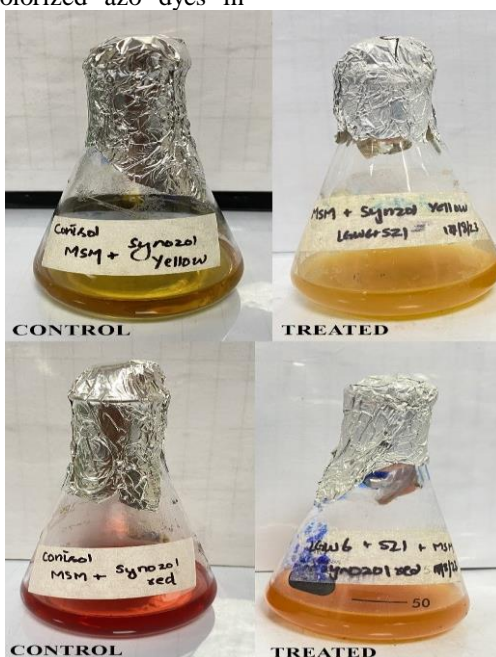
Figure 1. Decolorization of azo dyes by bacterial consortium LGW6 and SZ-1
